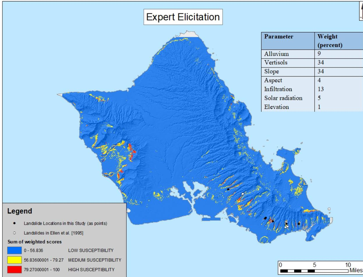
**Figure 36. Island-wide Slow-Moving Landslide Susceptibility Map with weights provided through Expert Elicitation.**
